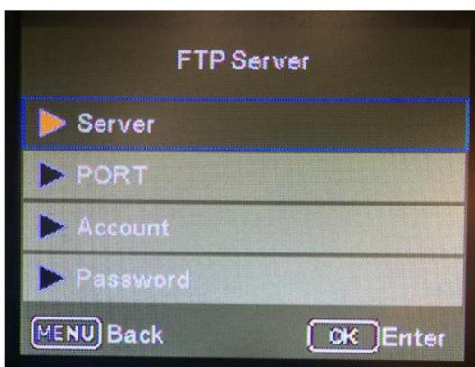
The File Transfer Protocol (FTP) is a standard network protocol that can be used for the transfer files between a camera and server via 4G network.
